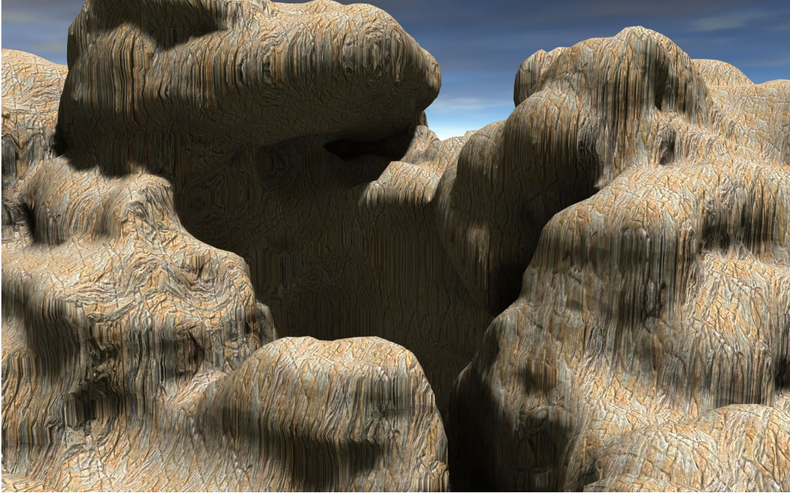
Figure 5.1. Texture coordinates obtained by projecting vertex positions onto the x - y plane exhibit severe stretching problems where the terrain surface is nearly vertical. The tangent frame on the undersides of the terrain features also has a reversed handedness.
